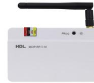
HDL MCIP-RF02.10 is a gateway based on IEEE802.15.4 standard MESH technology. Mesh Wireless Gateway has three communication interfaces: RJ45, HDL Buspro, RF, which can interconnect different media platforms (RS485, Ethernet, RF) of HDL intelligent devices .
