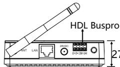
**24VDC:** Power supply, if the device connects to the HDL Buspro, it need not connect to DC power
