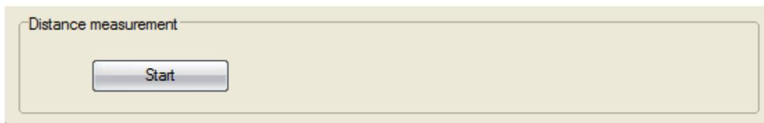
Click "Start" , the motor will measure moveable distance for the rail automatically, when it stops, will exit.
