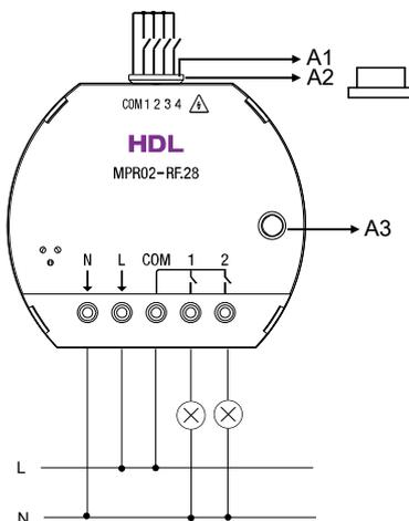
Figure 4. Wiring
