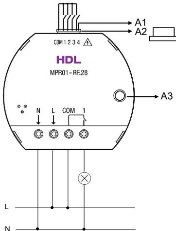
Figure 4. Wiring
